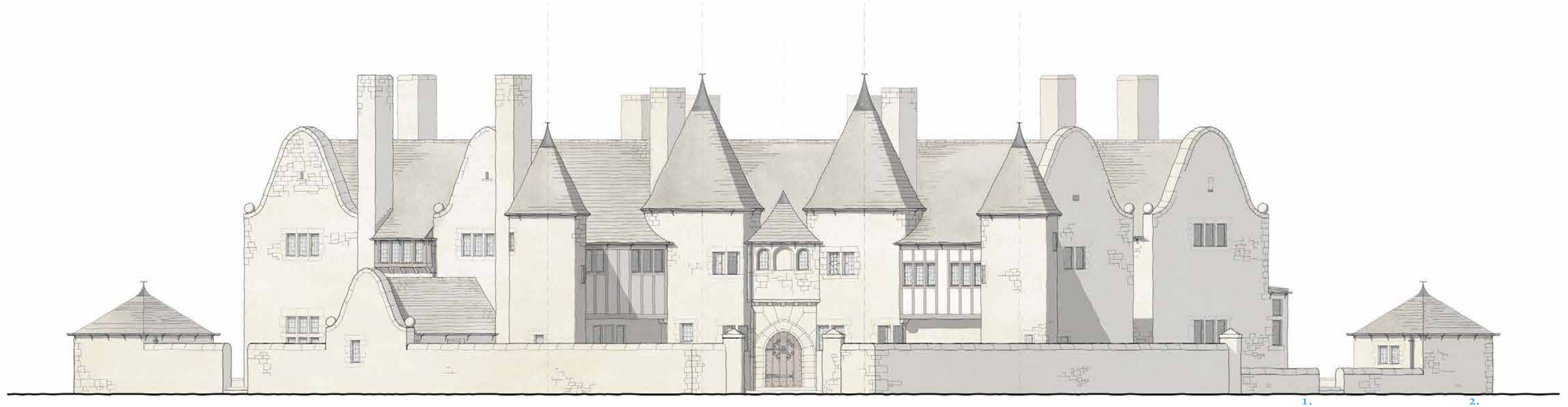
i. Proposed West Elevation by Yiangou Architects These are the painstaking created CAD versions of Baillie Scott's 1902 drawings - all now to a correct scale, and as accurate to the vision as we can be
