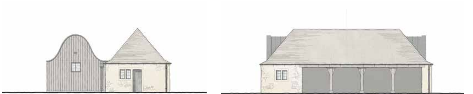
South west and south east elevations of proposed garage and plant room with bat loft and access
